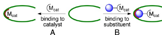
Scheme 10. Noncovalent ArM Formation via Binding (A) Directly to a Catalyst or (B) to a Ligand (blue)-Substituted Catalyst; Red Denotes Scaffold–Catalyst/Ligand Binding Interactions
